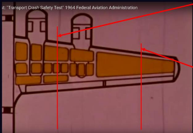
Inner wood pole impacts fuel tanks between engines
