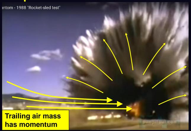
Momentum of the trailing air flow in the wake behind the plane creates the outward dispersion of the debris in all directions upon reaching the block.
