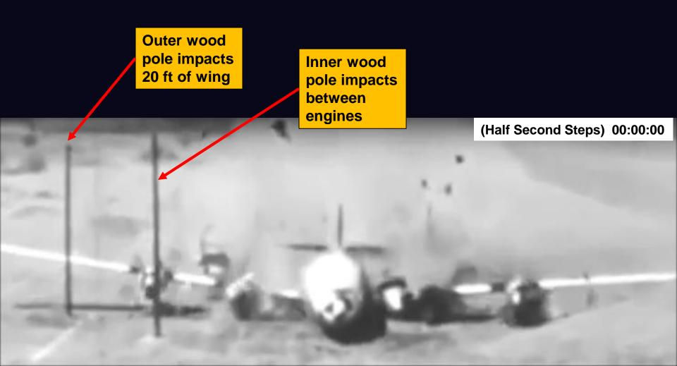
Outer wood pole impacts 20 ft of wing and fuel tank
